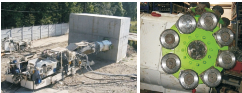
Fig. 7. A view of FR250 roadheader with new mining head with disk tools before the field tests
