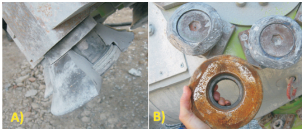
Fig. 8. A view of disk tool wear: A) made from steel type NZ3, B) made from ADI cast iron
