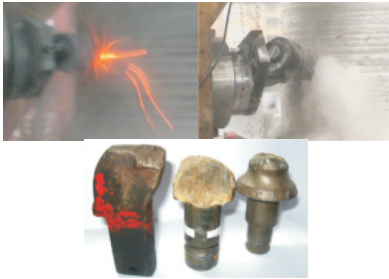
Fig. 2. View of frictional sparking and dustiness during cutting of a rock sample with a rotary-tangential pick and wear of pick wedge
