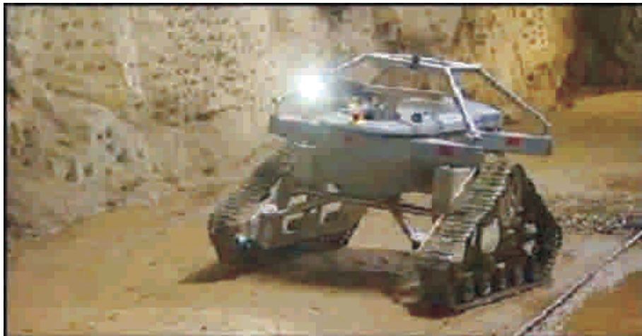
Fig. 8. View of 3D maps scanning robot
