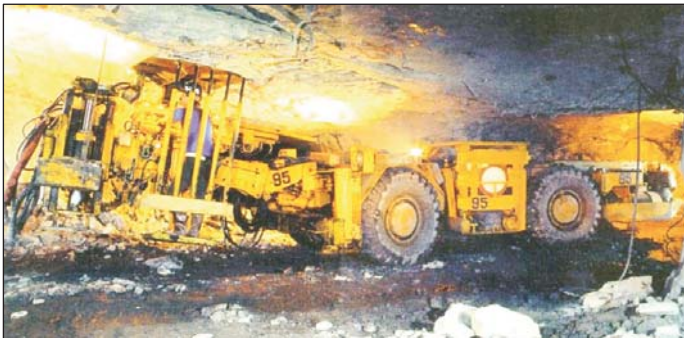
Fig 1. View of one of roof bolter operated in copper mines in Poland
