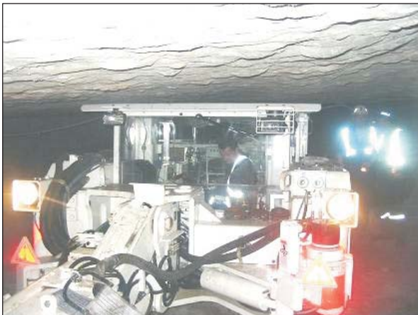
Fig 9. Roof Master 1.4 Automatic (view to the operator's end) during field tests
