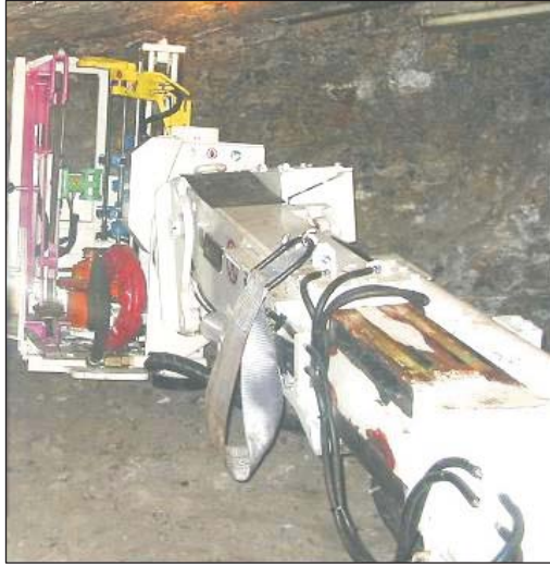
Fig 8. Automatic roof bolting head in Roof Master 1.4 Automatic during field tests
