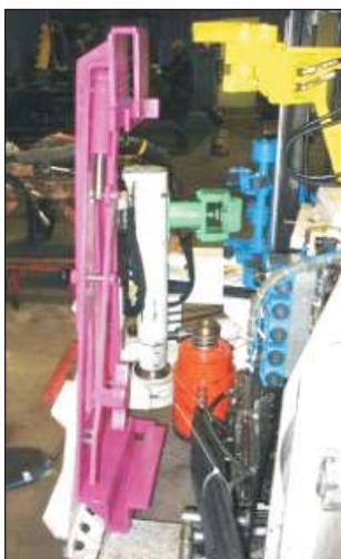
Fig 5. Automatic roof bolting head in Roof Master 1.4 Automatic - general view
